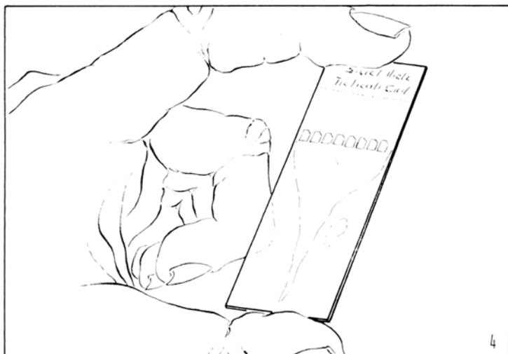
Fig. 4. Once 10 sections are aligned, the slide is tilted, forcing the water to run down slowly. If any section tends to run with the water, it can be repositioned by pushing it with the hair while there is still water on the slide.
